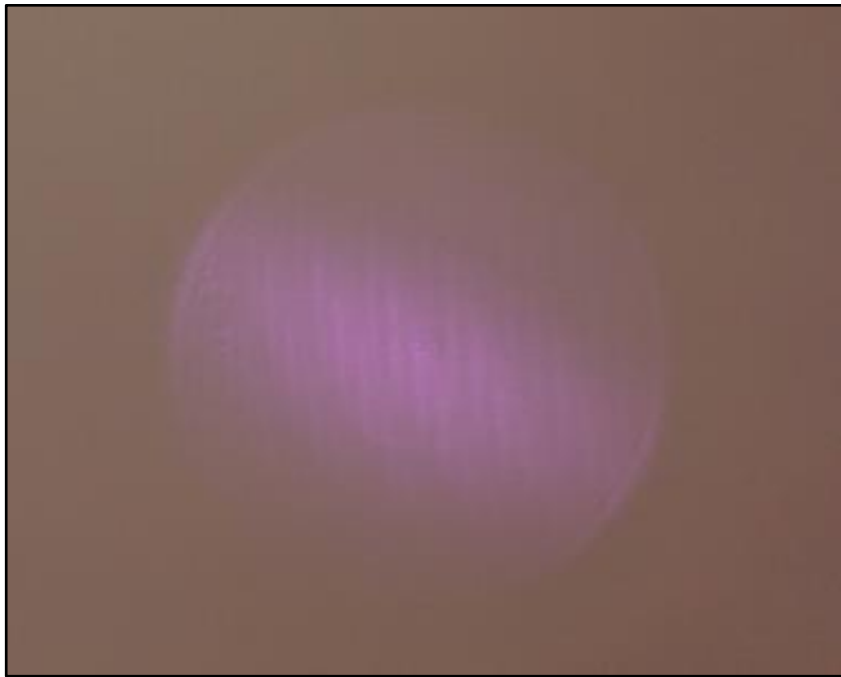
Figure 64: Spot Size using Spherical Lens and Thorlabs L904P010 905 nm Near Infrared Laser Diode (No Permission Needed)
