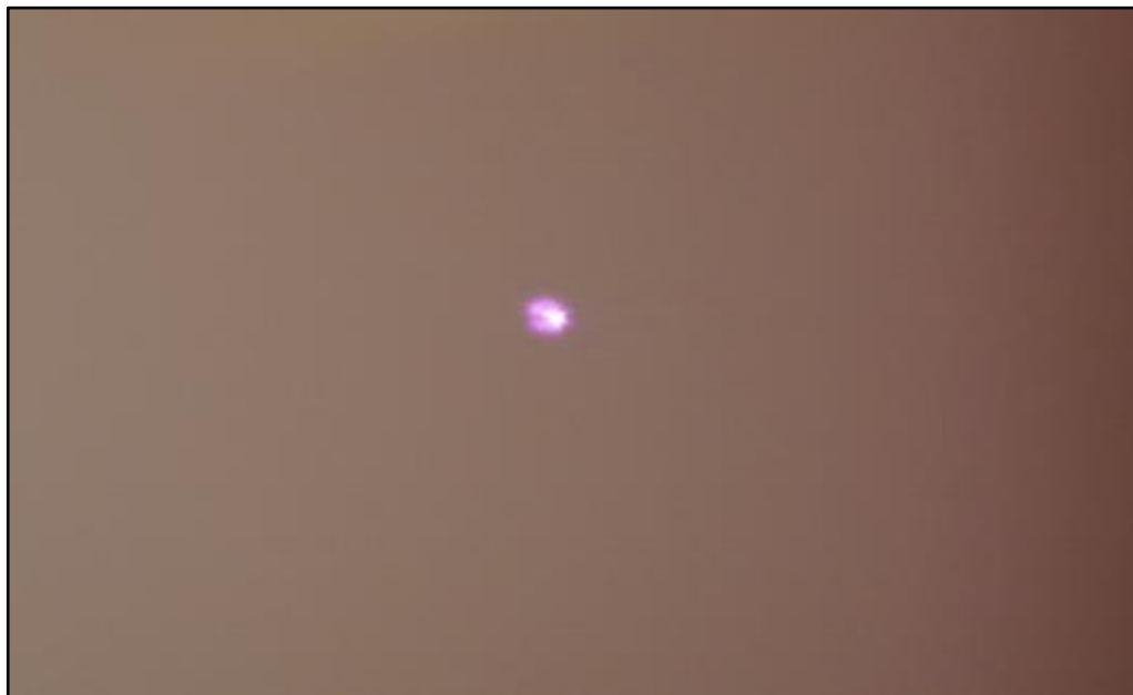
Figure 66: Spot Size using Plano-Convex Cylindrical Lenses and Thorlabs L904P010 905 nm Near Infrared Laser Diode (No Permission Needed)
